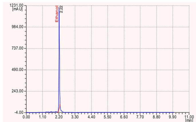
Fig2. G.C analysis of standard Ethanol
